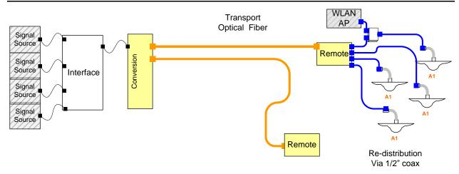
Like the active system, the hybrid system utilizes low-loss, fiber-optic transport and supports low-input power from the MNOs. This is a highly desirable feature, since it lowers the financial barrier for the MNOs. The passive part of the system supports the combining of various services at the remote hub location so that multiple services can be provided over a shared antenna.
