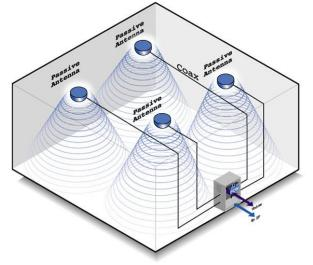
services being provided, obstructions in the coverage area, and the pattern of the antenna. For example, 4G technologies may require a denser antenna deployment than previous generations of cellular technology.
