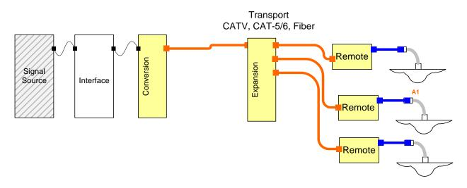
Active systems are best at providing coverage for a single MNO, grouping of MNOs, or grouping of services, such as cellular/PCS, and can be very cost effective. However, when a large number of MNOs or numerous services on a single MNO, such as cellular/PCS/LTE, then multiple "parallel" networks may be required. For a building, the actual design will be typically based on size, cost, output power, and antenna configuration option considerations.
