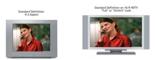
Figure 17: SD on 4:3 Monitor and 16:9 Monitor in 'Full' mode
