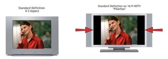
Figure 16: SD on 4:3 Monitor and 16:9 Monitor in 'Pillarbox' mode
